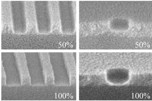
Fig. 2. Cross sections of 125 nm dense lines and contact holes in Cr absorber (roughly 32 nm on wafer level). The different overetch times (OE) for dense lines and contact holes as well as the strong etch bias is clearly visible.
