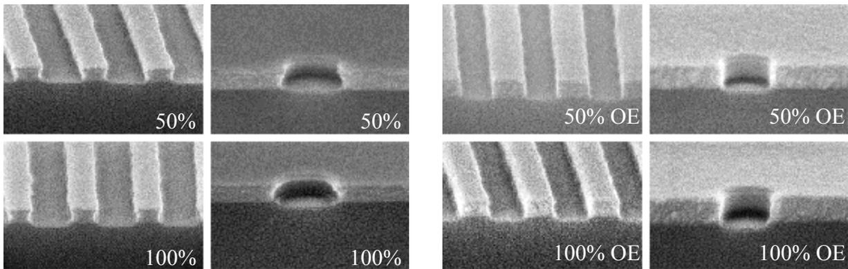
Figs. 3+4. Cross sections of 125 nm dense lines and contact holes in two different TaN absorbers (roughly 32 nm on wafer level). Although both materials show different side-wall profiles, they have a strong tolerance with respect to overetch time.
