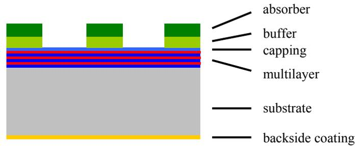
Fig. 1. Schematic cross section through an EUV blank.
