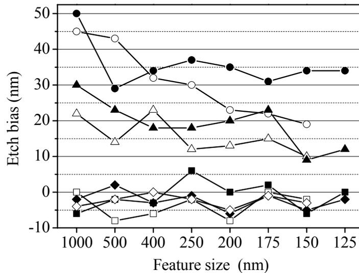
Fig. 5. Etch bias vs feature size for the various absorbers. The full symbols denote the values for dense lines, hollow symbols for contact holes (circles: Cr with 100% OE; triangles: Cr with 50% OE; squares: TaN with 50% OE)
