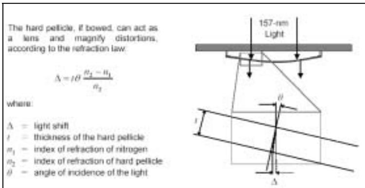
**Figure 7.** The figure shows how a bowed hard pellicle for 157 nm lithography can act as a lens and generate pattern placement error.
