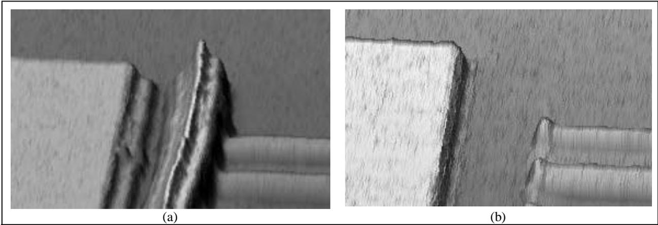
**Figure 4.** The figures shows a successful repair of a dark “killer” defect with the new RAVE nm650 nano-machining tool. The defect extends over almost 8  $\mu\text{m}$  in tight structures on a 70 nm customer tritone mask. (a): before repair. (b): after the nano machining process. Note also that the structure was brought into spec by additional FIB depositions.
