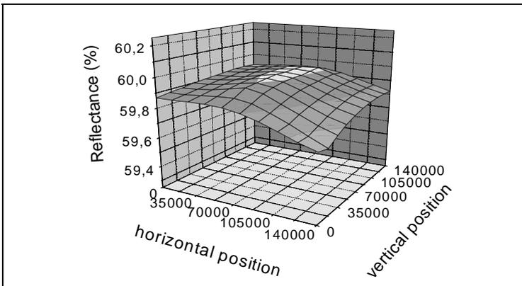
**Figure 10.** This figure shows the reflectance across the quality area of a patterned EUV mask. The measurements were performed at the synchrotron radiation beamline of the PTB at BESSY II and show a reflectance uniformity across the plate of less than 0.3%, which already fulfills the ITRS requirements.
