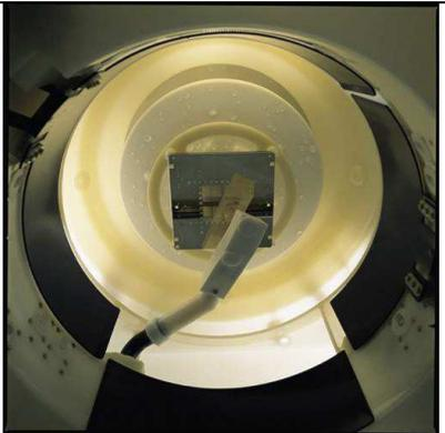
Fig. 2b Megasonic arm in process chamber
