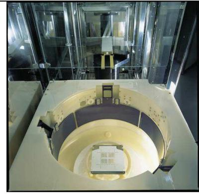
Fig. 2a View of Masktrack process chamber
