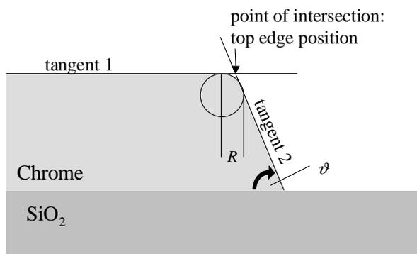
**Fig. 6** Definition of top edge position in the model. Tangent 1 terminates the upper plateau of the structure, tangent 2 is the edge slope tangent,  $\alpha$  the slope angle, and  $R$  the top corner radius. The point of intersection of the two tangents defines the top edge position.
