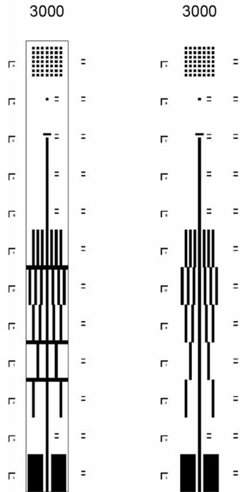
**Fig. 3** Layout of CD test structure group; black: quartz, white: chromium (top: clear structures, down: opaque structures).
