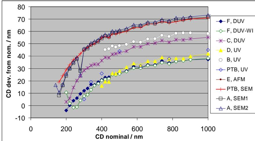
**Fig. 10** Round Robin measurement results on a COG mask standard for **isolated clear** line structures (the differences for the SEM results at nominally 280 nm structure are caused by a particle contamination).
