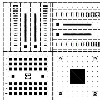
Fig. 2 Die layout of new mask standard.
