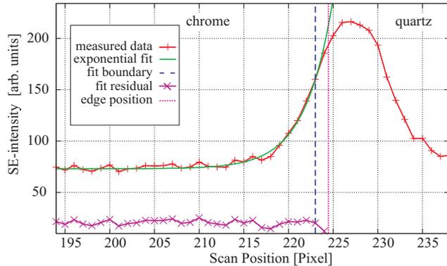
**Fig. 8** Experimental determination of top CD. An exponential function is approximated to the experimental data. The fit range is restricted to values below 65 % of the peak maximum, extrapolation to 100 % peak maximum defines the top edge position.
