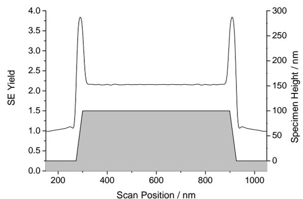
**Fig. 7** Monte Carlo calculated signal profile for an opaque 600 nm chromium line on quartz, edge slope  $80^\circ$ , no top corner rounding, e-beam diameter 10 nm FWHM, electron energy 1 keV (Note: the characteristic local minimum at the bottom usually is not detectable with EOMS system).
