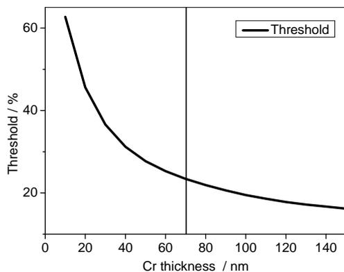
**Fig. 4** The influence of the thickness of the chrome layer on the threshold, calculated for homogeneous chrome.
