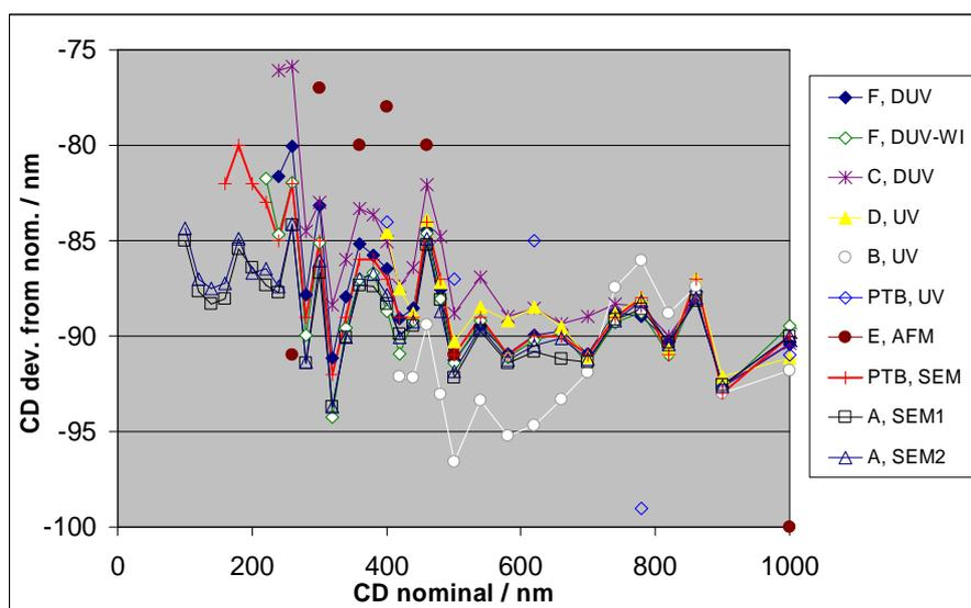
**Fig. 14** Deviations of all round robin results on a COG mask standard for **isolated opaque** line structures, CD offsets are referred to the width of structures between 820 nm and 1 μm as measured by the PTB SEM.
