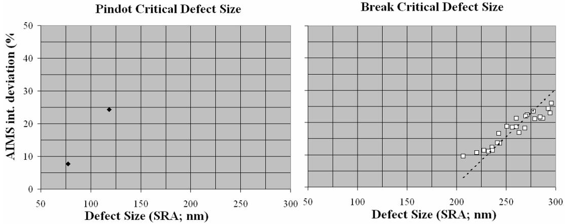
Fig. 5: AIMS intensity deviation with respect to the defect size of pin dots and line bridges (left image) as well as line breaks (right image)
