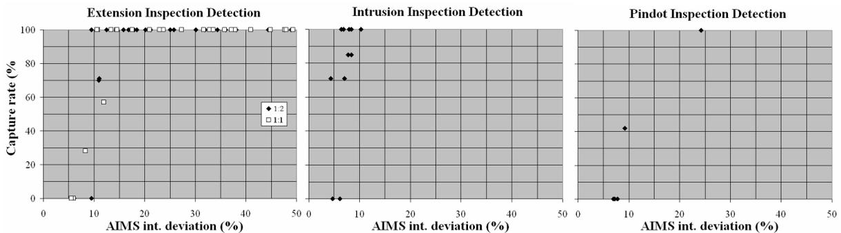
Fig. 7: Inspection capture rate with respect to the AIMS intensity deviation of extension with a 1:1 and 1:2 aspect ratio (left image), intrusions (middle image), as well as pin dots (right image)
