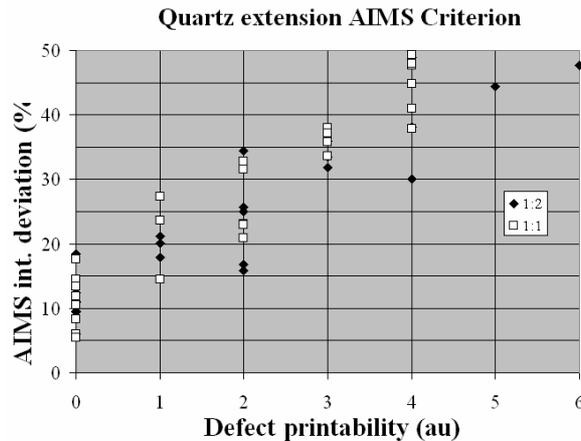
Fig. 2: AIMS intensity deviation plotted with respect to their defect printability of extensions with a 1:1 and 1:2 aspect ratio.
