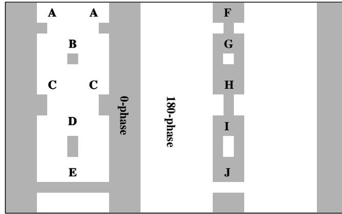
Fig. 1: Layout of programmed defects for a mesa-style de Cr-less PSM
