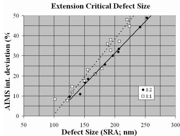
Fig. 4: AIMS intensity deviation with respect to the defect size of extensions with a 1:1 and a 1:2 aspect ratio
