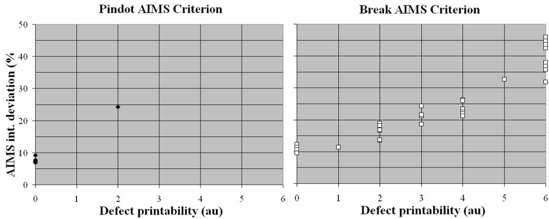
Fig. 3: AIMS intensity deviation plotted with respect to their defect printability of pin dots (left) and line breaks (right)
