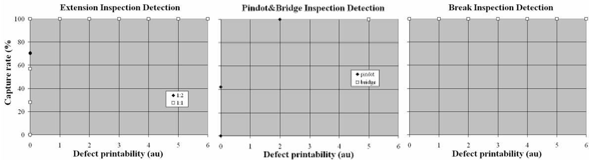
Fig. 6: Inspection capture rate with respect to the defect printability of extensions with a 1:1 and a 1:2 aspect ratio (left image), pin dots and line bridges (middle image), as well as line breaks (right image)
