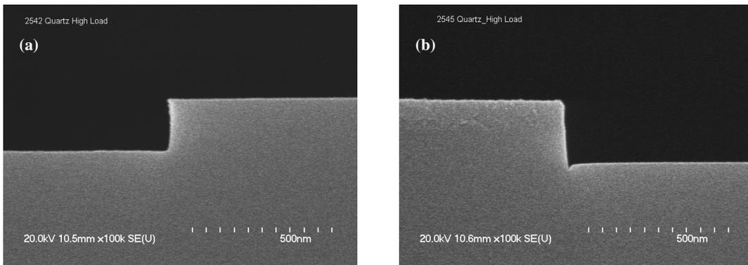
**Figure 5: Cross-section SEM Data showing (a) no micro-trenching (Cr stripped) and (b) large micro-trenching (Cr in image).**
