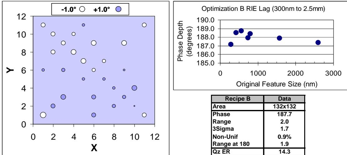
**Figure 8: Optimization Run B (High Source Power, High Bias Power, and Low Gas Concentration) resulting in 1.9° phase angle range (31 data points, 132x132mm<sup>2</sup>) and <2.0° RIE Lag (300nm to 2.5µm).**
