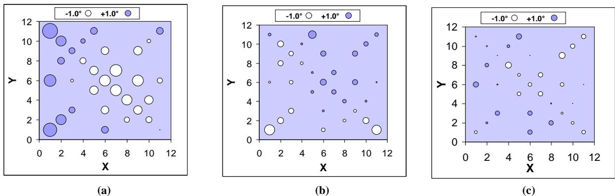
**Figure 2: Phase uniformity plots showing (a) center-slow etch footprint, (b) center-fast etch footprint and (c) best overall phase range ( $1.9^\circ$ ).**
