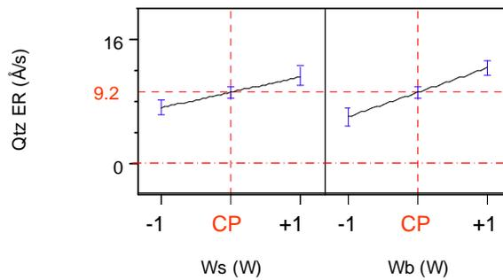
**Figure 3: Main Factor Trend Plots for Quartz Etch Rate.**
