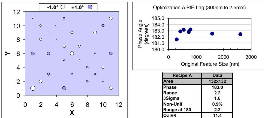
**Figure 7: Optimization Run A (Med Source Power, High Bias Power, and High Gas Concentration) resulting in 2.2° phase angle range (31 data points, 132x132mm<sup>2</sup>) and 2.0° RIE Lag.**
