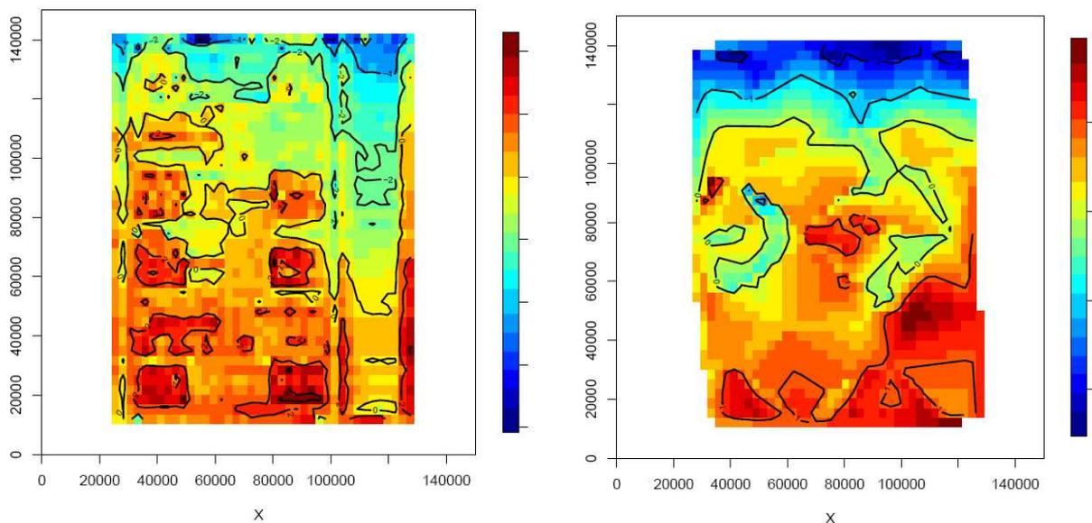
*Figure 1: Left) CD inspection report for dark lines in y-direction of a poly contact layer with several characteristic design solutions. Right) The same reticle measured by CD SEM. Due to lack of CD SEM measurement sites almost none of the subareas are resolved. The pronounced CD change in the upper edge is well visible and also the characteristic stripe on the right edge.*
