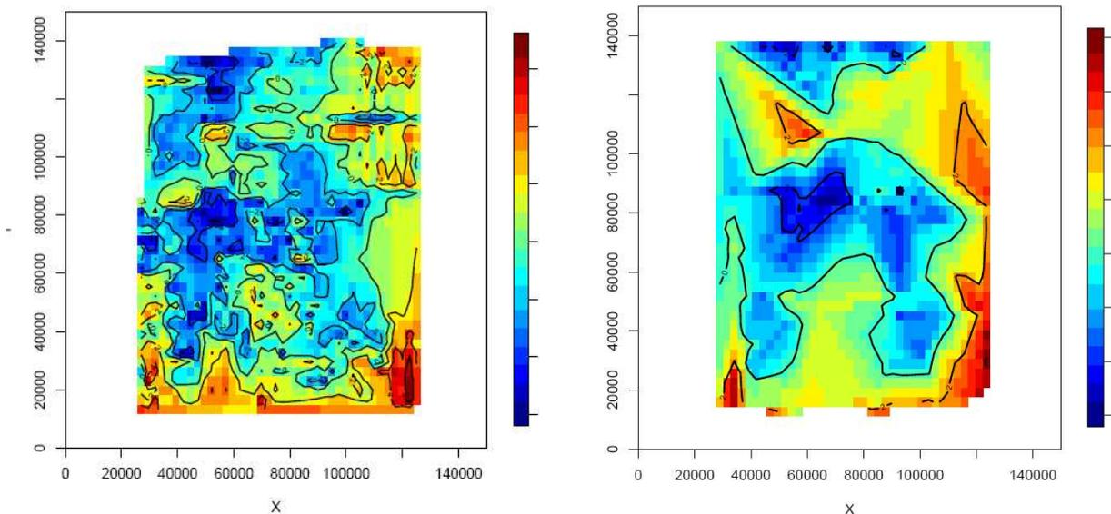
Figure 2: left) CD inspection report for dark lines in y-direction of a metal 2 layer with a characteristic lower right edge hotspot and middle left cold spot. Right) CD SEM report of the same mask.
