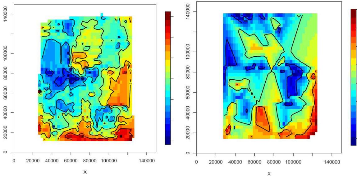
Figure 4: left) CD inspection report for dark lines in y-direction of a metal 4 layer of the same device as in figure 2 and 3. Right) CD SEM report of the same mask. These reports show the largest deviation, in particular in the upper edge and in the middle.
