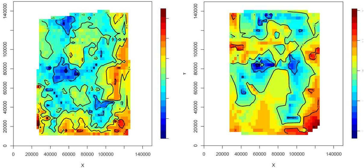
Figure 3: left) CD inspection report for dark lines in x-direction of a metal 3 layer of the same device as in figure 2. Right) CD SEM report of the same mask. The characteristic lower right edge hotspot and middle left cold spot are clearly visible, but not as pronounced as for the metal 2 layer. This can be seen in both reports.
