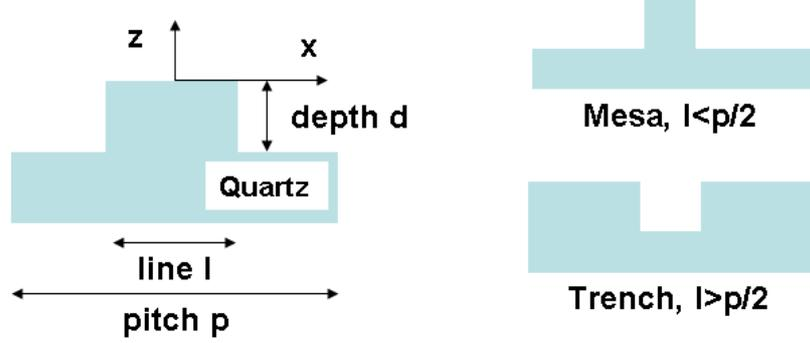
Figure 1: CPL mask: definition of geometry and coordinate system.
