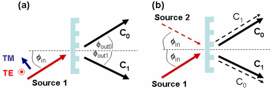
Figure 2: (a) illumination of dense lines and spaces with single source point (monopole) under an angle of incidence  $\phi_{in}$  and respective 0<sup>th</sup> and 1<sup>st</sup> diffraction orders with complex amplitudes  $c_0$  and  $c_1$ ; (b) dipole illumination with two individual source points located symmetrically to optical axis.
