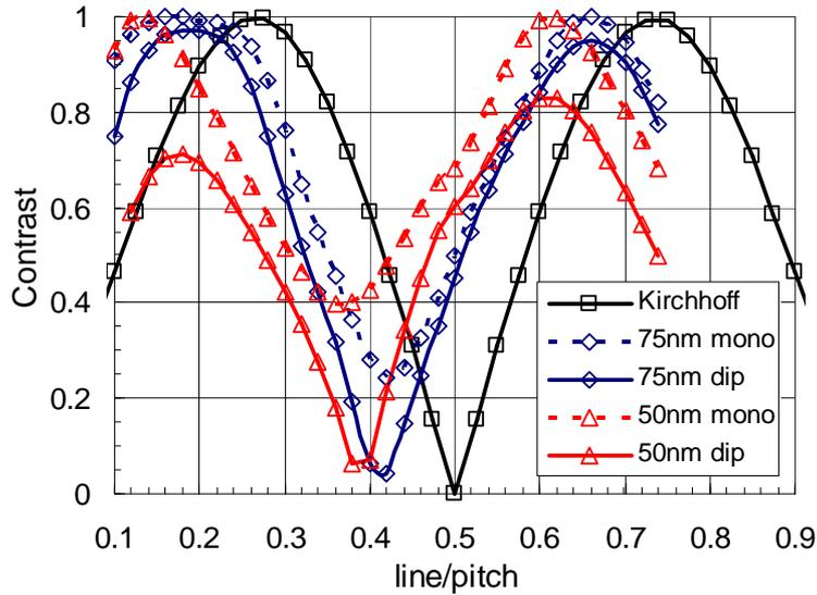
Figure 4: Image contrast for optimal monopole and dipole illumination according to Eq. (3) and (5), respectively (TE polarization, nominal depth for  $\pi$  phase shift  $d=\lambda/2/(n_{\text{Quartz}}-1)=171.4\text{nm}$ ). Whereas for monopole illumination the optimum contrast is obtained for smaller duty cycles, the phase error leads to image degradation for dipole illumination.
