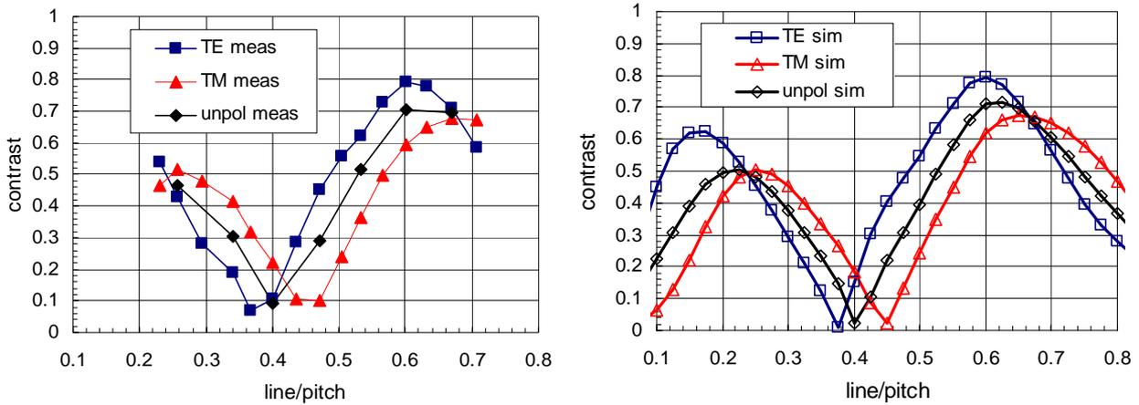
Figure 9: AIMS measured contrast (left) versus duty cycle for a CPL mask with half pitch 50nm compared to simulation results (right).
