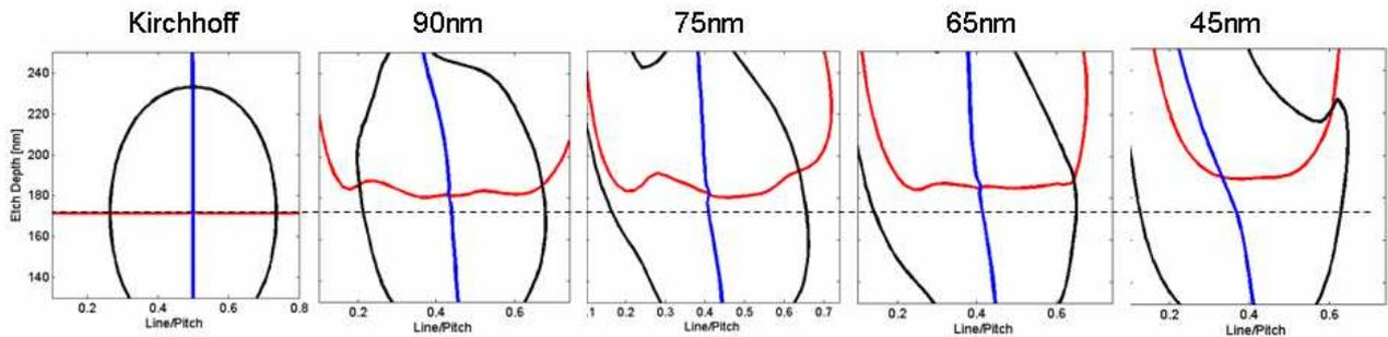
Figure 7: Evolution of contour lines for balanced structures according to Fig. 5 for varying pitches, also included is a comparison with a perfectly thin (Kirchhoff) mask, the dashed line corresponds to nominal etch depth; for half pitches smaller than 75nm mesa structures can not be balanced completely.
