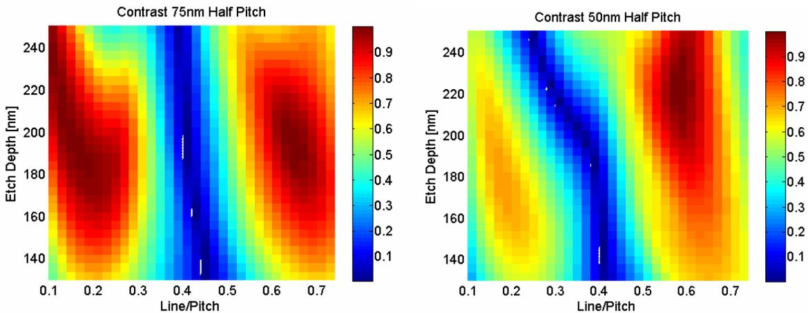
Figure 6: Image contrast for dipole illumination (TE) according to Fig. (5) for varying duty cycle and etch depth, respectively.
