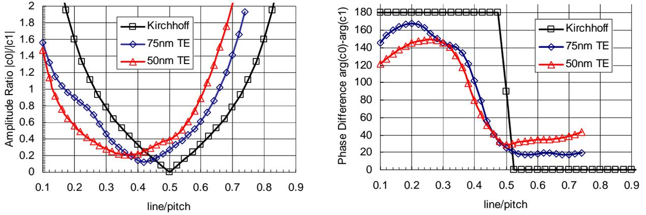
Figure 3: Ratio of magnitudes  $|c_0|/|c_1|$  (left hand side) and phase differences  $\arg(c_0) - \arg(c_1)$  (right hand side) of diffraction orders of infinitely thin mask (Kirchhoff mask) and a topographical mask (nominal etch depth  $d=171.4\text{nm}$  for  $\pi$  phase shift, optimal dipole, TE) for 50 and 75nm half pitch.
