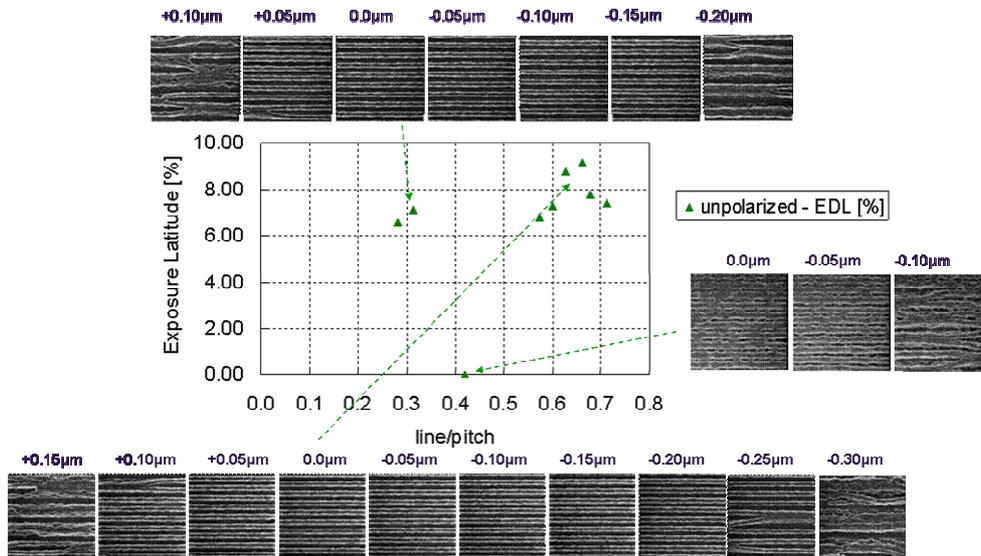
Figure 12: EL and DOF of 57.5nm lines-spaces versus the line-pitch ratio for unpolarized light.
