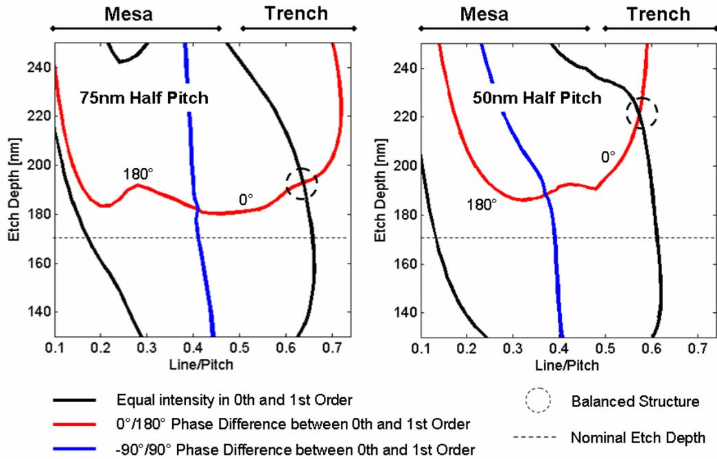
Figure 5: Contour plots for intensity and phase matching as a function of duty cycle and etch depth for 75nm and 50nm half pitch (TE polarization, optimal dipole); simultaneous balancing of intensity and phase is obtained for trench style structures only.
