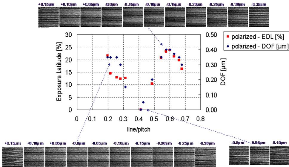
Figure 11: EL and DOF of 57.5nm lines-spaces versus the line-pitch ratio for TE polarization.
