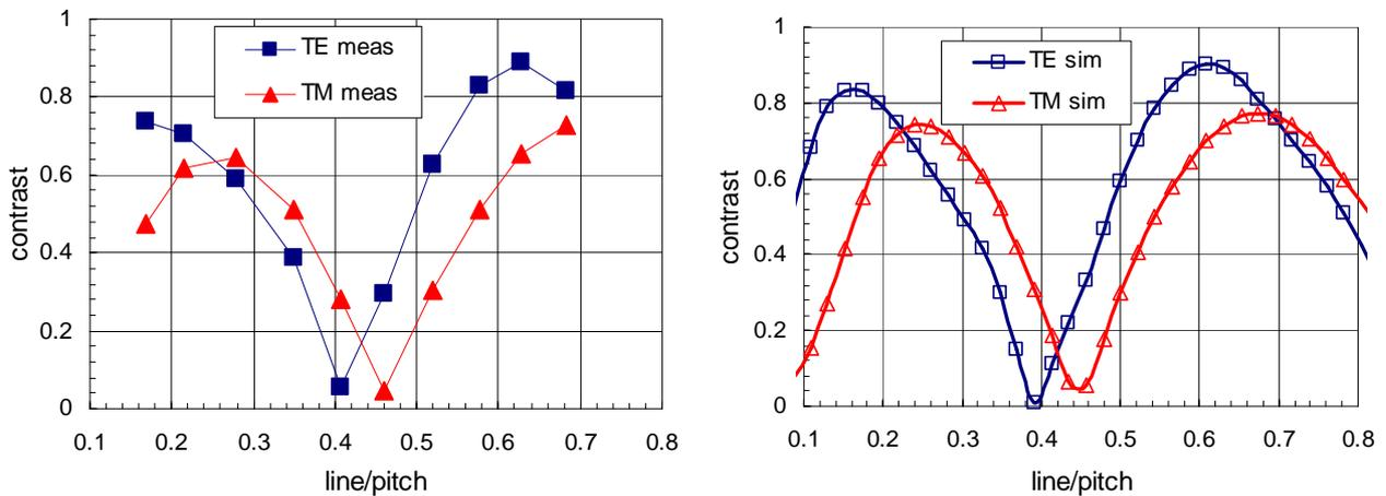
Figure 10: AIMS measured contrast (left) versus duty cycle for a CPL mask with half pitch 57.5nm compared to simulation results (right).
