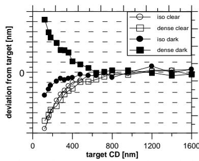
Fig.7 – CD linearity curves for iso-clear, dense-clear, iso-dark, and dense-dark features.
