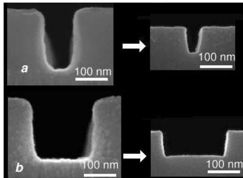
Fig.8 Comparison of the development of isolated space during the etch process. **a**, for small features **b**, for big features. Pictures on the left hand side show the side wall shape after resist development, picture on the right hand side show the side wall shape after Cr etch.
