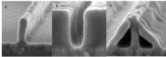
Fig.1 – shape of structures near resolution limit for **a**, isolated line **b**, isolated space **c**, dense lines and spaces
