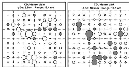
Fig.4 – demonstrates effect of directly-indirectly written feature - CDU comparison of directly (left) and indirectly (right) written features on positive resist type measured in resist. The dark features (indirectly written) exhibit slightly higher CDU due to shot placement error.
