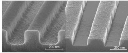
Fig.5 – LER as observed in SEM cross sections. Left picture shows the LER in resist, right hand picture demonstrates transformation of the resist LER into Cr layer.
