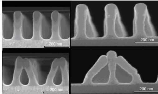
Fig.2 – Comparison of resolution limit for different resist thickness; on the left hand side the resolution limit at standard productive resist thickness of 200nm; right hand side resolution limit at 30% increased resist thickness. Upper row shows feature above the resolution limit – ca. 160 nm pitch for standard resist thickness, and ca. 240 nm pitch for thicker resist.
