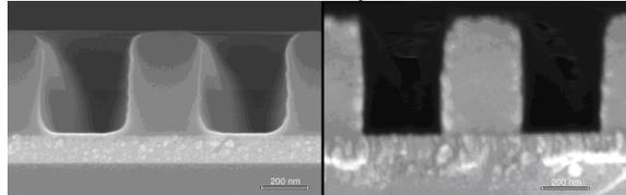
Fig.6 - Footing observed at positive CAR resist types due to poisoning of PAG on Cr surface - left. Barrel like side wall slope observed at negative CAR resists - right.
