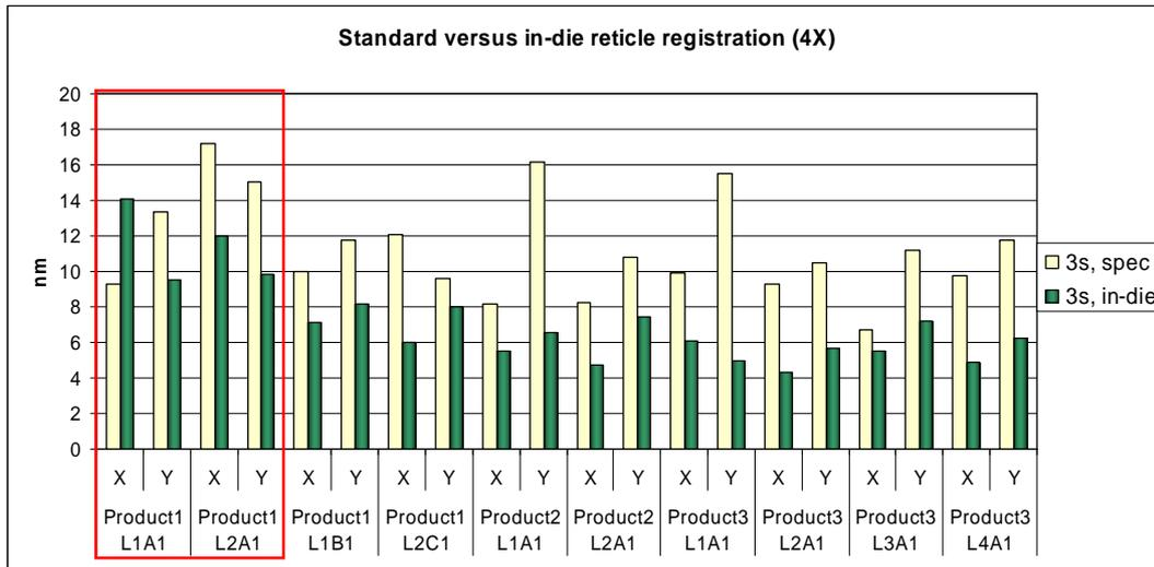
Fig. 4: Reticle registration results (4X) from different reticles measured on standard IPRO crosses and on in-die micro AIM targets as described.
