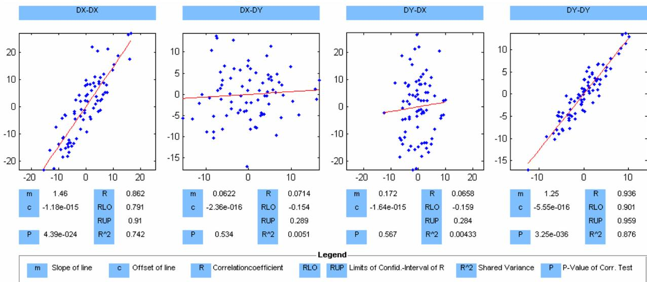
Fig. 10: Correlation of reticle registration overlay to wafer overlay (4X) for product 1 reticle set L1A1-L2A1.
