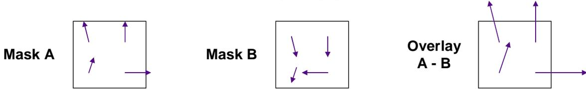
Fig. 6: Anti-correlated registration errors on mask A and B leading to the worst case of mask-to-mask overlay error.
