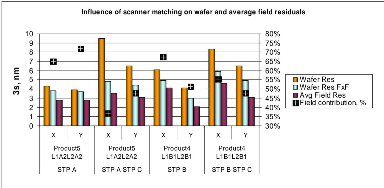
Fig. 12: Influence of scanner matching on wafer residuals for a composite field model (Wafer Res), a field-by-field model (Wafer Res FxF) and average field residuals (Avg Field Res).
