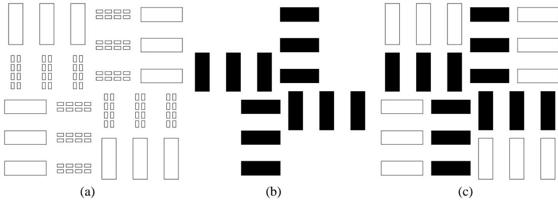
Fig. 2: Layout of micro AIM target: (a) simultaneous target layout for STI, (b) layout for poly gate, and (c) resulting micro AIM overlay target at poly gate. In black are the structures from poly gate, and in white are the structures from the STI layer.
