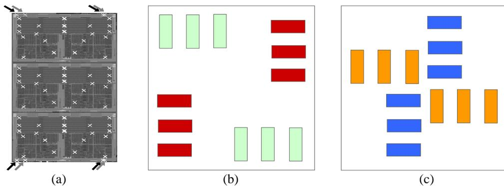
Fig. 3: (a) reticle registration measurement locations and schematic of micro AIM targets (b) outer and (c) inner features.
