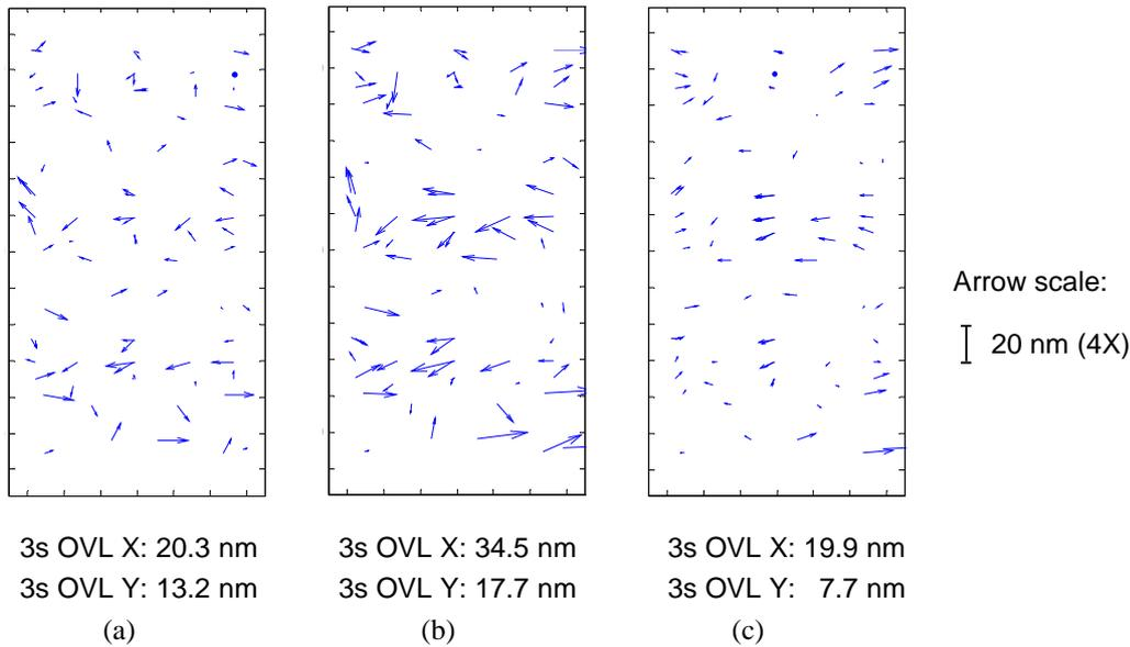
Fig. 11: Vector map of (a) reticle-to-reticle overlay, (b) wafer overlay, and (c) tool-induced distortions (same scale for all plots, 4X).
