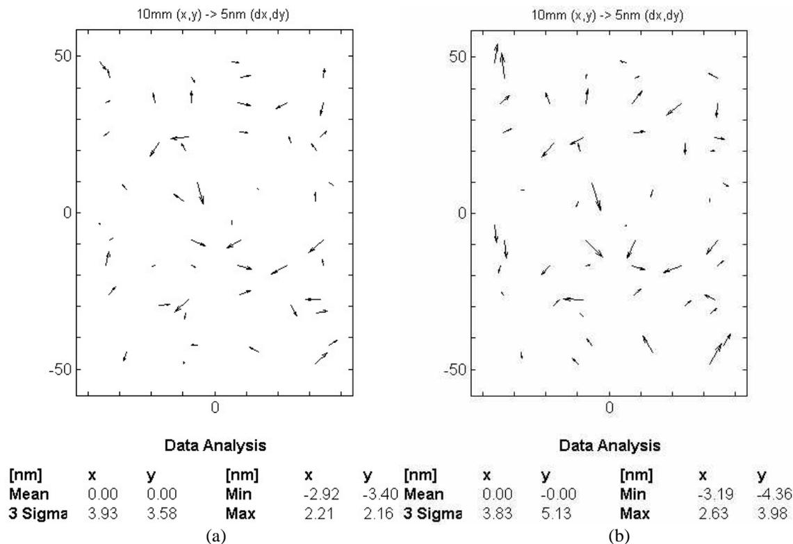
Fig. 7: Mask-to-mask overlay error introduced by different pellicles: (a) old pellicle set, (b) new pellicle set (4X).
