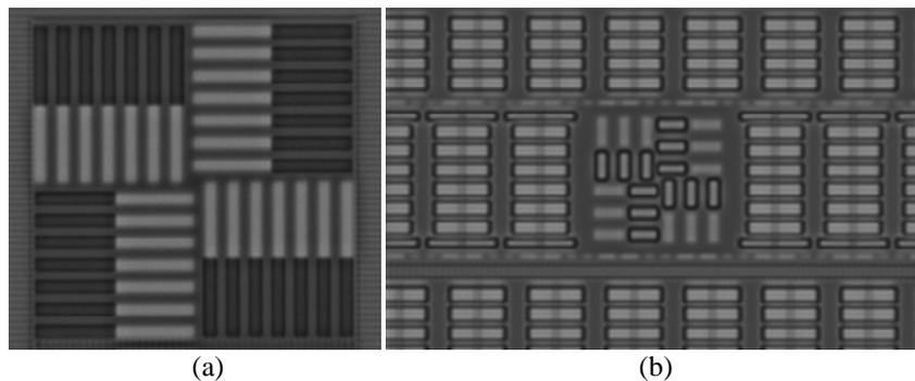
Fig. 1: Optical image of (a) a standard AIM, and (b) 3-bar micro AIM overlay target (FOV  $50 \mu\text{m}$ ).
