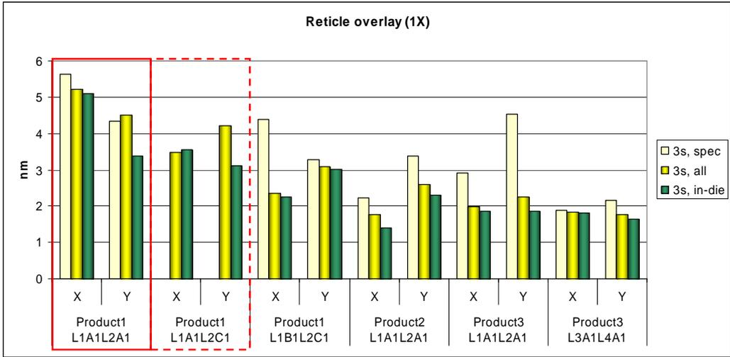
Fig. 5: Reticle-to-reticle overlay (1X) results from different reticle pairs measured as specified (spec), on all standard and micro AIM targets (all), and micro targets in-die only (in-die).
